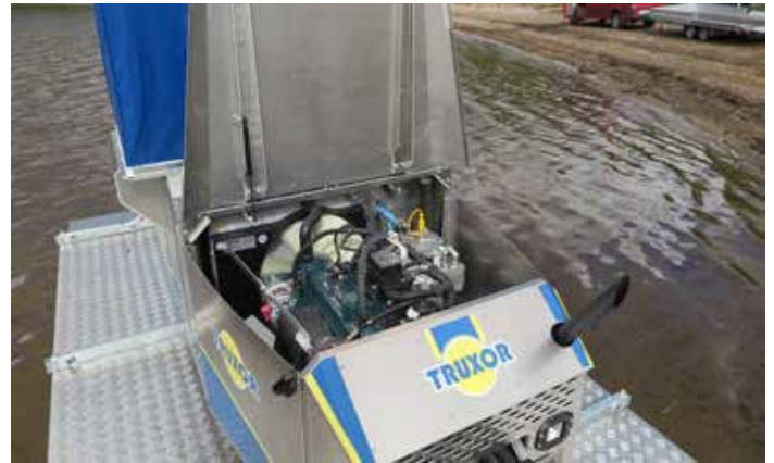
Easily accessible engine compartment facilitates service.
