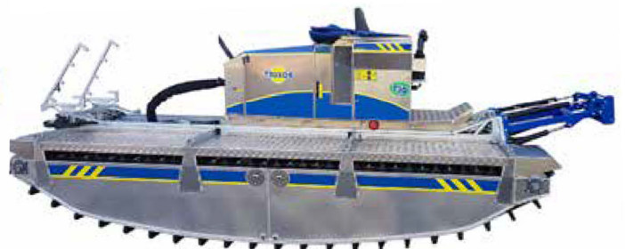
The movable driver's cab is hydraulically adjusted and works as counterweight during heavy lifts in water.
